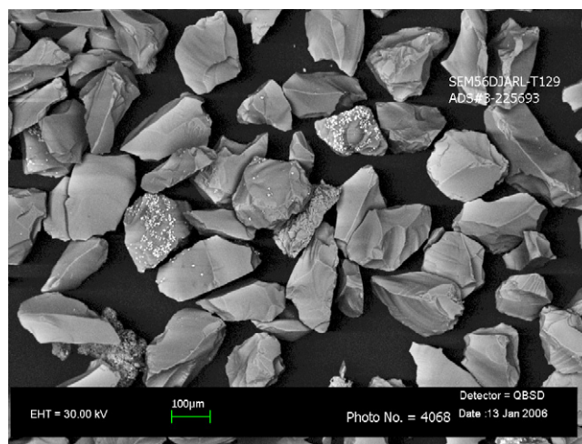
Fig. 6. SEM micrographs of 56-day leached Pu LaBS glass showing crystalline PuO 2 inclusions and no observable alteration phase formation.
